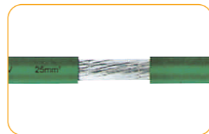
Piercing effect of wire core
